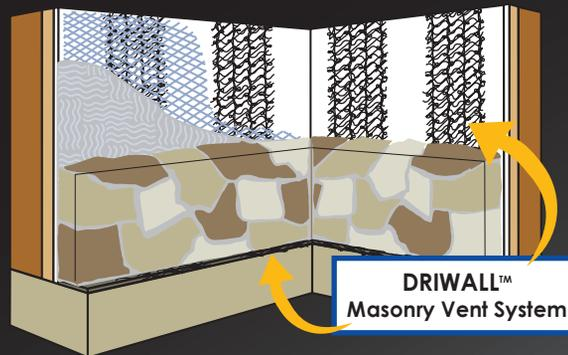
**DRIWALL Masonry Vent Strips** are the most economical solution for draining and ventilating masonry walls. The product creates a vertical ventilation strip approximately every two feet along the wall. That strip is allowed to exit the wall at the bottom creating the path for liquid moisture to drain and for air to circulate.
